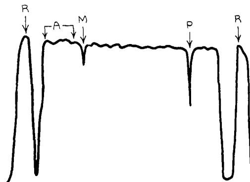
Fig. 3.—Sedimentation equilibrium of precipitated lysozyme in 0.8 molal cesium chloride and 3.6 molal ammonium sulfate at 59,780 r.p.m. in the AN-D rotor. The protein appears as a single prominent spike near the bottom of the centrifuge cell.
